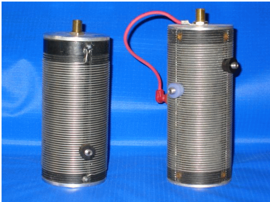
Prototype 80 meter coils 48 turn coil on the left 52 turn coil on right.
